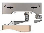
The limitations on the striking angles are the same as for an indirect roller lever, with a limitation on speed of 2 m/s.
